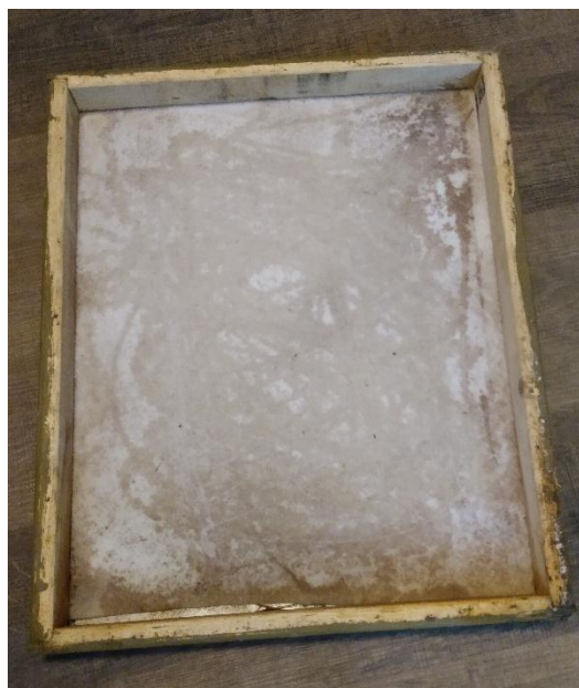
This well-used fume board is made from 1x2 lumber, felt and metal flashing. Neither craftsmanship nor aesthetic appeal are required!
