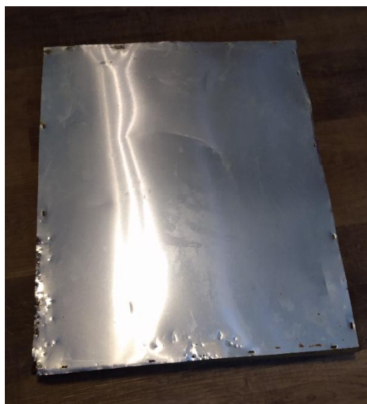
This well-used fume board is made from 1x2 lumber, felt and metal flashing. Neither craftsmanship nor aesthetic appeal are required!
