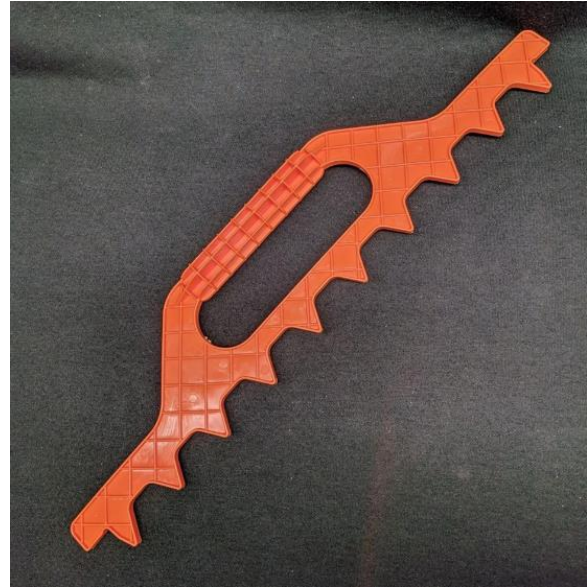
A 9-frame spacing tool makes it easy to spread nine frames evenly in a 10-frame box. A 7-frame version is available for use with an 8-frame box.
