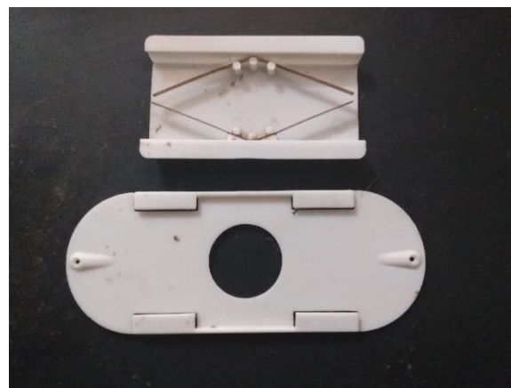
A disassembled Porter Bee Escape, showing the springs that allow a bee to leave but not reenter. The device fits perfectly into the center hole of an escape board aka inner cover.
