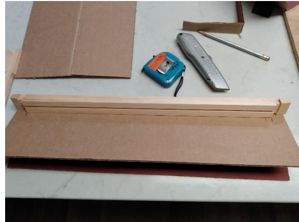
It is a good idea to use a frame to ensure that the dimensions are correct.
