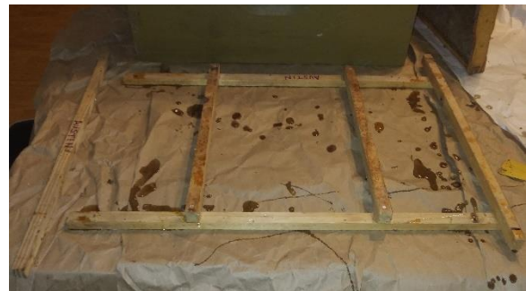
A frame popper. The two central rails fit within the inside dimensions of the box so they pop frames from the super when the super is pressed down. After extracting, the super can be positioned so that it rests on the longer rail on the far right and the free-standing stick on the left; this supports the entire box in an "unpopped" state and makes refilling it with empty frames easier.
