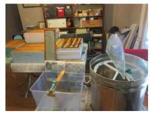
My extracting "assembly line" is carefully arranged to reduce motion and the chance of honey spills. From the top left are full supers, the super being emptied, my uncapping tank and my 9-frame motorized extractor.
