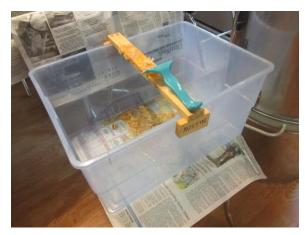
My homemade uncapping tank features a sturdy platform for resting the end of a frame.
