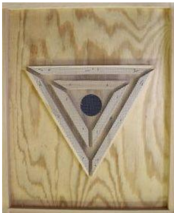
Triangle bee escape. The triangle is covered with wire mesh. Bees enter the maze from the honey supers via the hole in the center. By following the walls, all routes lead back to the outside.
